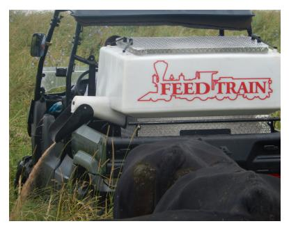
The Feed Train UTV feeder is an ideal tool to replace bucket feeding. Capacity is 600 pounds of shelled corn, which will unload in less than two minutes. The tank is translucent so feed level is visible. The 4" auger services several different types of feed including cubes. Auger height is designed to fill any type of feed bunk.
